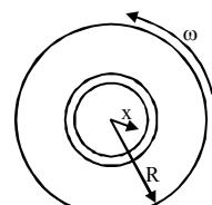
Current due to this ring  $dI = \frac{dq}{T} = \frac{\sigma 2\pi x dx}{2\pi} \omega$
